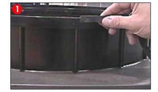
2 Apply the tape all the way around the edge and cut off any excess.
